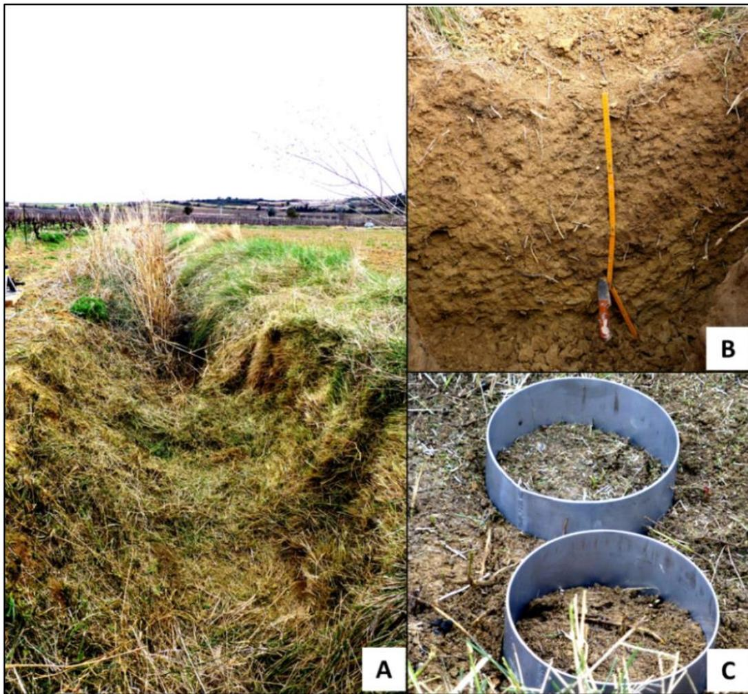
**Figure 4.1-1:** *A: studied ditch near the outlet of the Roujan catchment. B: soil profile underlying the ditch bed. C: core sampling.*
