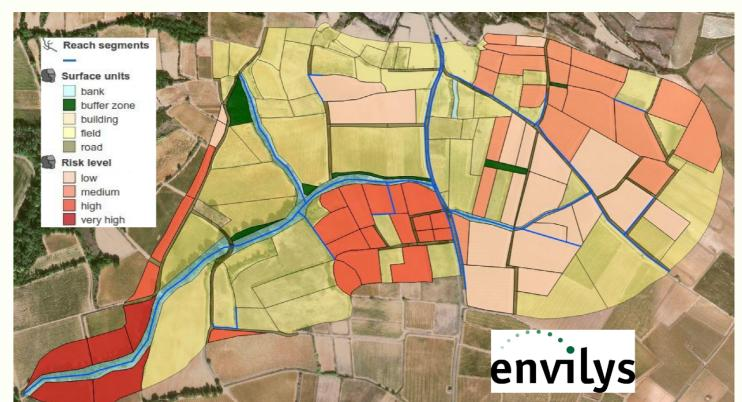
units (fields, roads, banks, buffers) and 40 reach segments (ditches, pipes, rivers). The coupled model is made of hydrological models and fate-and-transfer pesticide models.
